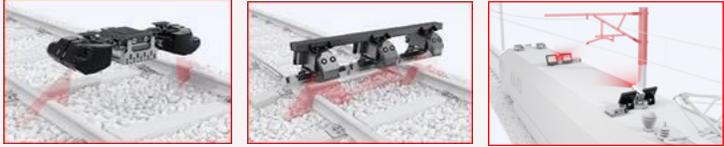
Catenary / Pantograph defect detection
